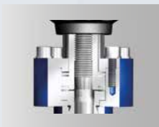
Optimal handling: Non-rising handwheel (PN 63-160)
