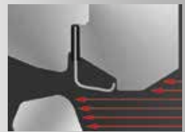
Extended service life because the metal sealing ring is protected against negative flow effects.
